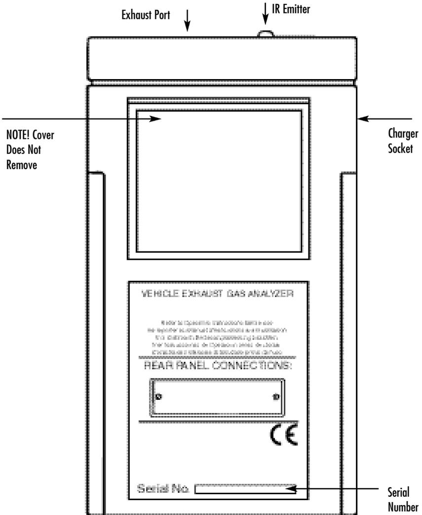
**\*Note:** DO NOT cover exhaust port as this will severely affect analyzer operation
